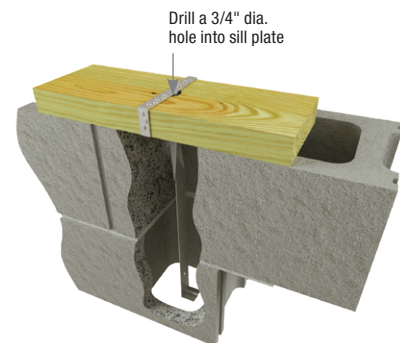
Alternate ST2-TZ installation with 3/4" center hole in mudsill
